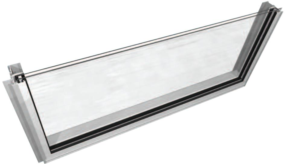
The Series 8100 Fixed Window has a 4-1/2" (114 mm) deep frame designed to match typical building conditions, including our entrances and storefronts. An efficient thermally insulated frame accepts 1" (25 mm) glazing. Available in an array of architectural coatings and anodized finishes.
